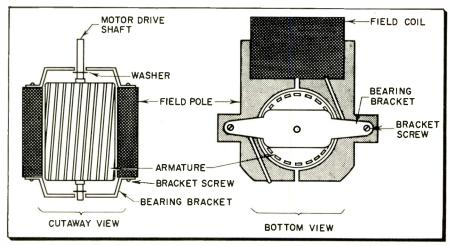
bracket, to hold the armature in position as firmly as possible
