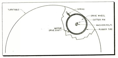
Fig. 3A-Flat and identation on drive-wheel tire. B-Removing tire from drive wheel.
