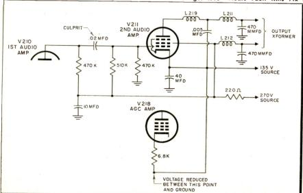
Schematic of section of Du Mont RA 164-5 chassis in which leaky audio coupling condenser killed pix and sound by reducing the 135v source voltage. (See "Audio Fault Kills Pix")
