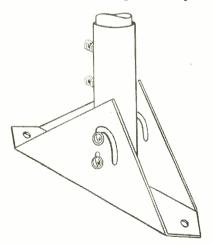
tioning of the mast. Mast and antenna are set in the base, then "walked up" to the vertical position and locked. South River Metal Products, South River, N.J.— TECHNICIAN
