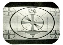
Fig. 2—Insufficient picture height, vertical linearity approximately normal. Possible sources of trouble: Loss of emission in the vertical oscillator or sweep amplifier; increase in value of oscillator (multivibrator) plate resistor; defective vertical output transformer; improper plate or grid voltages on output tube; loss of capacitance in the vertical amplifier cathode bypass condenser.
