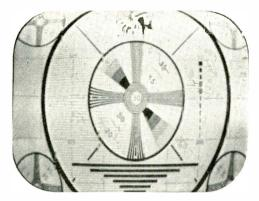
Fig. 4—Excessive height. Usually caused by excessive "drive" at grid of vertical amplifier. Check for decrease in value of charge resistor in plate circuit of vertical ascillator; reduced capacitance in charging capacitor; defective height control.
