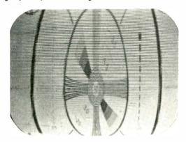
Fig. 5—Excessive height, vertical linearity poor, foldover at bottom of raster. Possible sources of trauble include: Leakage in the coupling capacitor between the vertical oscillator plate and amplifier grid; loss of capacitance in the oscillator's charging capacitor.
