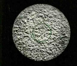
Microscopic look at the cathode surface reveals soft, even texture, necessary for efficient tube performance
