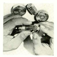
9-pin straightener, mounted back to back. The compact device may be carried in the tool box or in a pocket. CBS-Hytron, Danvers, Mass.—TECHNICIAN
