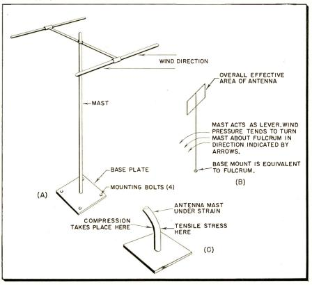
assume that the overall area of the antenna assembly exposed in any one direction is one square foot. At the base of a thirty-foot mast, the 20-pound per square foot wind pressure produces a torque of 600 footpounds. If this mast is set in a steel plate on a concrete base, the minimum safe stud-type expansion bolt diameter is  $\frac{3}{4}$  in.
