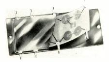
Triple-tie cross-over filter, model UV-3, employs a printed circuit to eliminate the need for two down leads when both a UHF and VHF antenna are in operation. Use of one down-lead eliminates interaction between the UHF and VHF systems, in addition to simplifying the installation job. Impregnation before encasement to make the unit moisture-proof and fungus-proof also eliminates possibility of drift or shorting of components. TV Products Co., Springfield Gardens, N.Y.— TECHNICIAN
