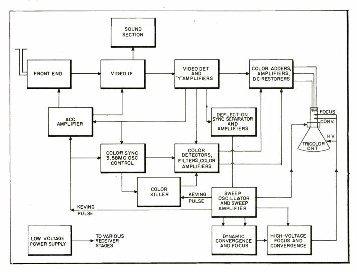
"Y" signal is the luminance information of the color signal—that is, it contains information regarding the brightness of each pictorial unit. This "Y" signal is, incidentally, the only one of the several video signals present in the color transmission that a monochrome set will also respond to, and is equivalent to a monochrome video signal.
