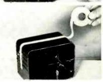
Cement Co.) and then it was firmly placed in original position. Adhesive tape was then used around the entire case to hold the broken piece in place until the cement had set.—H. Leeper, 1346 Barrett Ct., NW., Canton 3, Ohio.
