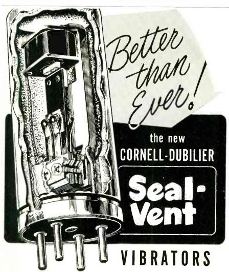
★ You'll agree that this is the greatest advance in vibrator design in the past 17 years. This new CORNELL-DUBILIER vibrator is SEALED until used, to prevent oxidation of the vibrator contacts, and VENTS itself when needed! Heat generated when the vibrator is put into service melts the wax out of the sealed vent and permits air circulation . . . for LONGER LIFE and EVEN GREATER PERFORMANCE!
