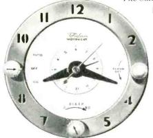
Used as an alarm clock, this C-57 Telechron clock-radio timer automatically switches radio on at preset time. Approximately 10 minutes later insistent alarm sounds to make sure heavy sleepers wake up. The "sleep switch" enables you to drift off to sleep with music—the radio shuts off automatically later. Many clock radios have an outlet that turns on electric appliances any time up to 10 hours after setting.
