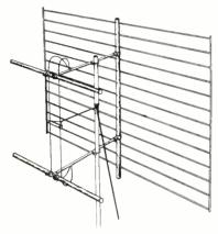
the low band, shorted stubs across the dipole elements lower the fundamental resonant frequency and at the same time provide a good impedance match on the low channels. These stubs are quarter wave resonant on the high band and therefore have negligible effect upon high band operation.—Gonset Company, Burbank, California.—RADIO & TELEVISION RETAILING.
