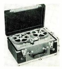
be rewound during operation. The Magnemite operates from self-contained dry batteries which last 100 hours without replacement. At the tape speed of 1% inches per second with a frequency response to 3000 cycles, two full hours of recording time can be accommodated on a single 5 inch reel. A complete description, including specifications and price may be obtained by writing to: Amplifier Corp. of America, 398 Broadway, New York 13, N. Y.—RADIO & TELEVISION RETAILING.
