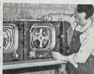
Spot-Check Functional Test "Final line" sets selected at random for operational check.
