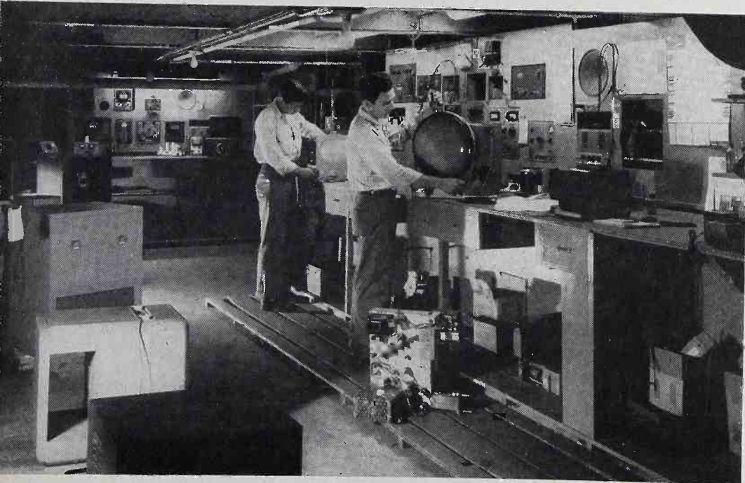
This roomy, well-equipped service department (below) has separate benches for radio and for TV work. The technician at the right is testing for high-voltage at the picture tube.
