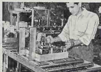
Severe Vibration Test "Shake Table" checks stability of all wiring in the chassis.
