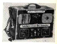
use of a station signal off the air. The generator is connected to the set at the antenna terminals and may be tuned in by using the regular channel selector. Sold through jobbers for \$39.95 by Superior Inst. Co., 227 Fulton St., N. Y. 7.—RADIO & TELEVISION RETAILING.
