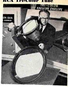
E. W. Engstrom, vice-president in charge of research for RCA Laboratories, explains the RCA tri-color television picture tube to a group of television manufacturers. He is holding a cut-away model of the 16 inch tube, which RCA is turning over to its licensees with complete manufacturing details. Below is RCA's newest 21-inch tri-color tube, which will afford the largest direct-view color television pictures ever seen. vision pictures ever seen.
