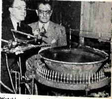
Watching the glass to metal cone sealing operation of General Electric's 24-inch cathode ray tube are Dr. W. R. G. Baker, right, vice-president and general manager of the Electronics Department, and J. M. Lang, left, manager of the Tube Divisions.
