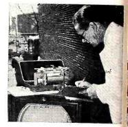
ON AND OFF 140,000 TIMES! Another eye opener for your customers! Even the *switches* are LIFE-TESTED ... turned on and off 140,000 times, equal to *years* of home usef
