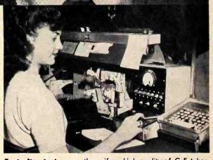
Test after test assure the uniform high quality of G-E tubes. Here G-E receiving tubes get a factory "short" test. Later comes an electrical-characteristics check; also tests for noise, microphonics, life, appearance, gas, air, and hum. G-E tubes perform better because they are better!
