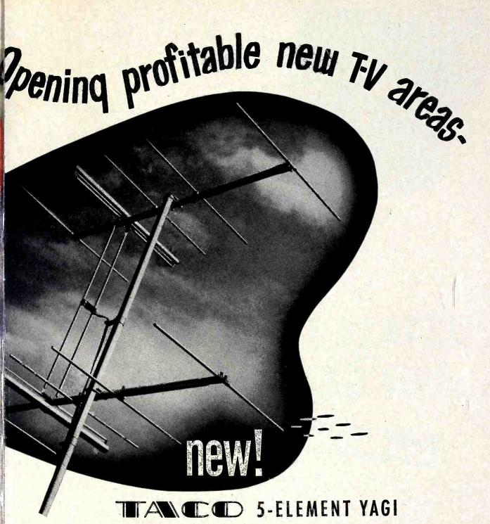
OPENS TV sales areas beyond present limits. Picks up where 4-element antennas leave off in fringe area reception. Extra director steps up gain and minimizes interference. Two-diameter antenna element increases bandwidth.
