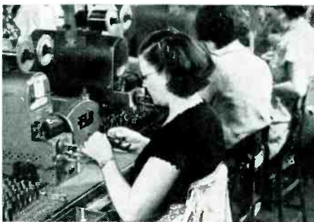
In manufacturing tuner coils , as shown above, much of the work is done by hand due to the fine and delicate parts assembled. Yet at Philco's plant at Croydon, Pa., coils are turned out at the rate of 150,000 a week.
