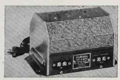
dial. It is not necessary to switch from low to high bands. Regulation of gain is made by tuning the receiver contrast control. No need to re-tune after the booster warm-up period. Signal drift is eliminated. Uses four 6J6 RF tubes. Power consumption: 20 watts. Power source: 105-125 volts, 50-60 cycles. AC Input: 150-300 ohm twin lead. Output: 150-300 ohm twin lead. Size: 7¾" x 5½" x 434", Net weight: 4 ibs. Lists at \$49.50. Electro-Voice, Inc., Buchanan, Mich. RADIO & TELEVISION RETAILING.
