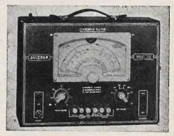
power factor from 0 to 60%. Ranges from .00001 to 1000 mfds. in 4 steps. Jackson Electrical Instrument Co., 18 South Patterson Blvd., Dayton 1, Ohio.—RADIO & TELEVISION RETAILING.
