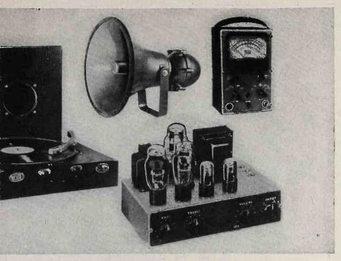
Typical component units which might make up the assembled "kit" used to take the measurements described in the text. Two loudspeakers are shown, a cone and a horn, but the one actually used should be a duplicate of that which is recommended for the PA job. The signal source, amplifier and meter could conceivably be all combined in one chassis.
