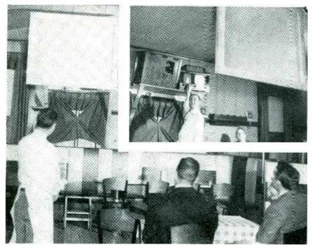
Fig. 2—Front and (inset) rear views of the hanging screen in Ahern's Restaurant, Ansonia, Corn. The 3x4 foot translucent screen may be viewed from either side. Inset: Francis Ahern tunes his direct-view receiver, which "feeds" the projection unit, shown at the left of the receiver.
