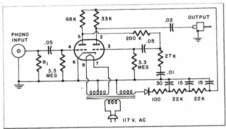
Fig. 3: Pre-amp and equalizer for G.E. variable reluctance pickup. R-1 is chosen for desired high frequency response characteristic. Typical values are shown in the text.
