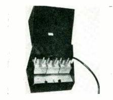
is composed of three coupling units, each of which feeds two TV sets, a power supply, and a mounting cabinet. More than six television receivers may be operated from the same antenna by connecting additional PD-16 assemblies in series. The equipment has been standardized for 52 ohm coax. When 300 ohm line is used, model MT-11 impedance matching transformer may be used. Lynmar Engineers, 1721 Delancey St., Philadelphia 3, Pa.
