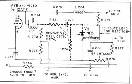
Fig. 3—Removal of DC restorer, G.E. models 12T3, 12T4, etc.
