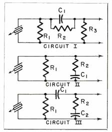
Fig. 2: Basic equalization circuits for crystal pickups which may need attention when new unit is added. Response is explained in test.
