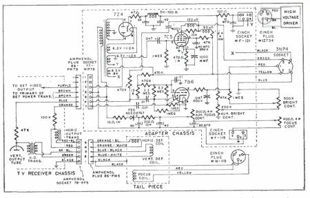
Fig. 1—Schematic of the adapter unit. The 10 connections to the receiver chassis are at plugs 86-PM7S and 78-PF5. "High voltage driver," "3NP4 socket," and "Tail piece" are parts of projection unit. The adaptor, described in the text, is shown in fig. 6.
