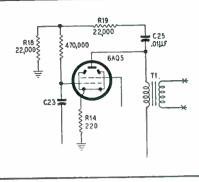
Fig. 7-Audio Output Circuit
