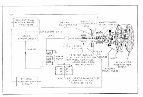
Fig. 1—Artist"s conception of the RCA single gun tricolor kinescope, with block diagram of components needed for its operation. "R, B, G" refer to red, blue and green.
