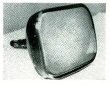
which permits the use of a single field ion trap. The tube has a useful picture area of approximately 140 square inches. The 19inch tube (19AP4A) has a useful picture area of about 250 square inches. Further information on these two new tubes may be obtained from the Tube Division of the General Electric Company, Schenectady, N. Y.
