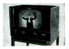
phono attachment, features a rectangular flat face tube. Cabinet used had previously been used for 12½-inch models, but is now adaptable to the 16-inch chassis by employing the rectangular tube. List price in mahogany is \$299, blonde wood is higher. Also available with Dumont Imputuner, full FM radio and Sightmirror for \$339. Match-
