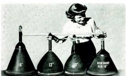
As shown above, the new 16GP4 16-inch metal kinescope is 5% inches shorter than the previous 16-inch tube (16AP4) and is actually shorter than 10- and 12-inch tubes. Shortened length was made possible by the use of 70 degree deflection. The RCA "Filterglass" face plate provides improved contrast.
