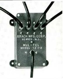
One of three types of distribution units available in the Brach Mul-Tel System. For a 4-set system the cables on the top connect directly to TV sets; in a 16-set system each wire feeds into another distribution unit which in turn supplies 4 sets. Cable on the bottom is 72-ohm coax from the antenna. Provision is made for use of 72 or 300 ohm downlead to any input. (Pat. applied for)
