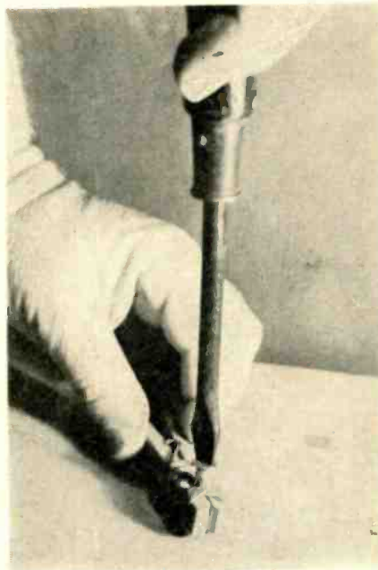
Fig. 2—Spring-type clothespin saves fingers when starting screws and short nails.
