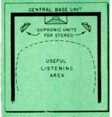
Fig. 6—System shown takes advantage of open-back satellite-type speaker enclosures to provide increased sound dispersion.
