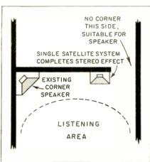
Fig. 4—Ar original monophonic speaker system is converted for stereo use by adding two satellite speakers. The center speaker carries bass frequencies of both channels.
