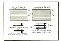
Fig. 1—The development of quarter-track tape doubles playing time offered by halftrack tape and brings pre-recorded tape prices into closer competition with records.
