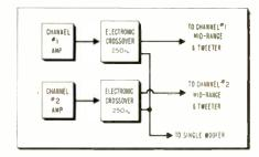
Fig. 5—Crossover networks inserted between the amplifiers and speakers removes the bass component from each channel and directs it to the system containing the woofer.
