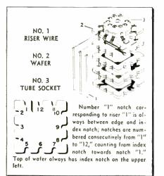
Fig. 1—Correct module mounting is simplified by a notch between risers 1 and 12.
