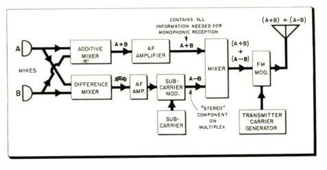
Fig. 1—The sum and difference technique supplies all the information needed for monophonic listening to the main carrier. The sum signals modulate the main carrier, while the difference signals, with one signal reversed in phase, is impressed on the subcarrier.
