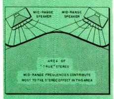
Fig. 1—This basic speaker placement approach provides a wide stored listening area in large racms. Placing speakers parallel to the listener would necessitate closer spacing to achieve the proper effect.
