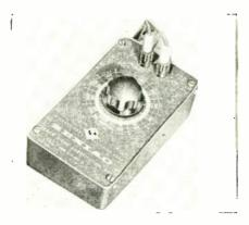
decade-type substitution box contains a selector switch enabling interchange of any one of the 11 component diodes. The original Model A, 1-watt Zeniac and the new 10-watt Model B Zeniac are now available. International Rectifier Corp., 1521 E, Grand Ave., El Segundo, Calif. (ELECTRONIC TECH-NICIAN 9-26)
