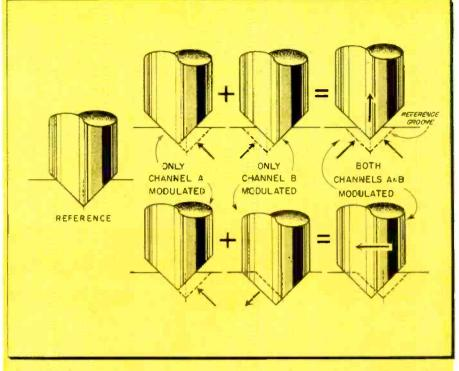
Fig. 3—Stylus may move up, down, right or left, depending on information impressed on sidewalls. Sidewalls are modulated by the net result of each channel's signals.
