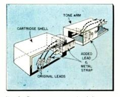
Fig. 1—To convert a two-pin shell to accept a stereo cartridge, it is necessary to provide a connection for the third terminal.
