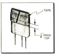
Fig. 2—Wrapping the top of a transistor with tape facilitates handling the component in almost inaccessible areas of small radios.
