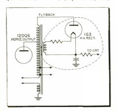
in inductive components, both electrically and mechanically, make it impractical to maintain a complete stock. Substitution, therefore, is usually eliminated as one of the two methods of checking a horizontal output transformer (H.O.T.) since it is normally not stocked. Because of this, replacement of H.O.T.'s presents many difficulties.
