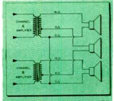
Fig. 5—Establishing a third channel. While this doesn't add anything to bass response. It does imprave directional sense with respect to the center of the program source.
