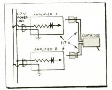
Fig. 3—Some a-c/d-c equipment and cartridges may present a possible shock hazard.
