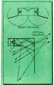
Fig. 3—The single "satellite-type" speaker carries the frequencies above 300 cps from one channel. The larger speaker carries bass frequencies of both channels plus all other frequencies of one channel.
