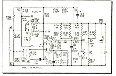
Fig. 4—The voltage regulator circuit illustrated has a 300 v d-c input between terminals 6 and 9. The tube socket and most of the components are on the module shown in Fig. 28.
