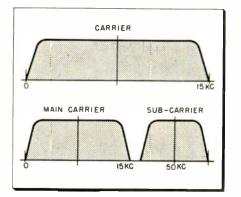
Fig. 3—Restricting the deviation of the main programs leaves room for one or more subcarriers to carry additional programs,
