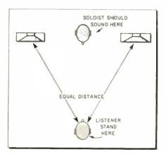
Fig. 2—A soloist's voice should appear to come from the center when the speaker outputs are properly phased and balanced.
