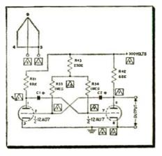
Fig. 7-Low-level video signals are amplified by the circuit shown. A single pentode is used. The module is shown in Fig. 2E,
