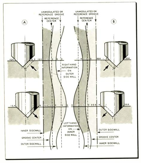
the Westrex 45/45 system uses the principle of diagonal movement, i.e., both a lateral and a vertical movement with a 90° relationship to each other, with the vertical and horizontal axis rotated  $45^{\circ}$  as shown in Fig. 1.
