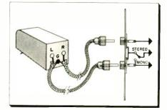
Fig. 2—The hum-free switch shown enables the user to revert to monophonic playback.
