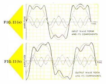
Since envelope delay is defined as the derivitive of phase with respect to frequency, exact measurement of envelope delay is difficult. In practice, however, envelope delay may be approximated by the following definition:
