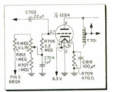
Fig. 2—Missing filement socket pin No. 4 cut the heater voltage in half and resulted in insufficient current flow. The inadequate current affected the TV set's height.
