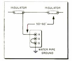
Fig. 2—A low-directivity antenna is usually satisfactory for reception on all bands.
