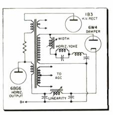
Fig. 3—A defective external circuit such as the damper, yake, width, etc., can load down the circuit and kill the high voltage.
