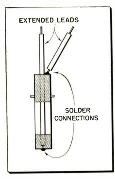
Fig. 1—Modified "twist-lock" fuses, as shown, will enable the technician to measure current without removing the TV chassis.
