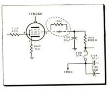
Fig. 3—Inserting a 120 ohm resistor in the 17DQ6A's screen grid of RCA series 800 TV sets will remedy parasitic oscillations.
