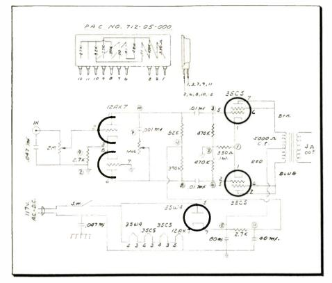
Fig. 8—The amplifier circuit shown uses a flat-type module with 12 connections. The module connections are noted on the schematic by corresponding circled terminal numbers.
