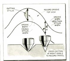
Fig. 4—The sidewise motion of the cutter results in a narrower groove with respect to the playback stylus whenever the groove is laterally modulated. The narrower groove pinches the stylus, causing it to rise and fall. Since stereo cartridges reproduce the vertical component as well as the horizontal one, lateral modulation increases distortion in the vertical component.
