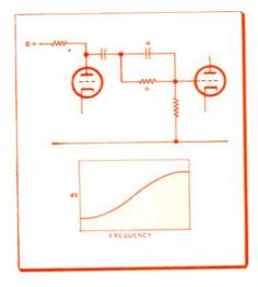
Fig. 5—A simple equalizing circuit to produce a low frequency slope, depending on the circuit values of components with asterisks.
