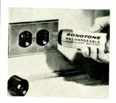
directly into any 110-volt a-c outlet. An overnight recharge is sufficient. The cartridge slips easily into any flashlight now using "D"-size cells. No adapters are needed. 12 different sizes of cells are available; is rated at 4.2 ampere hours; the smallest is rated at 75 ma hours. All sizes are 1.25 volts. Cartridge price: \$7.95. Sonotone Corp., Elmsford, N. Y. (ELECTRONIC TECHNICIAN 8-26)
