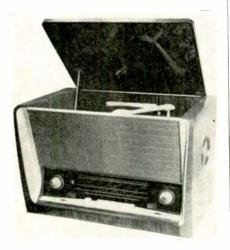
The "Latvia" table model radio-phono combination made in USRR is designed to receive standard broadcast, FM and short wave. Note "German styling."
