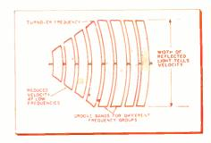
Fig. 4—Constant velocity cut discs appear as shown when grooves are held to a light.
