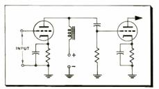
Fig. 3—Schematic diagram shows triode vacuum tube connected for grid-leak detection.
