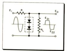
down voltage, the counterpart of vacuum tube inverse peak voltage, occurs when voltage is sufficient to break through the diode's barrier region and become a conductor. However, the barrier region may heal itself when the excess inverse voltage is removed, whereas a vacuum tube would probably be permanently damaged by arcing between plate and cathode. The breakdown voltage of a zener diode is dependent on the resistivity of the silicon itself.
