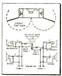
Fig. 1—Position of doors may be varied to affect sound pattern of each channel. Variable resistors shown are tweeter brilliance controls and midrange presence controls.
