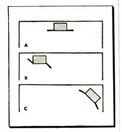
Fig. 3—Reflector door may be adjusted to accommodate positioning in room.
