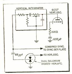
Fig. 1—Defective horizontal afc selenium dual diodes affect the vertical sync section.
