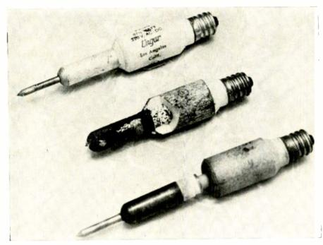
The lower two tiplets have been damaged through improper removal and inadequate maintenance. In order to prevent oxides from freezing the tip into the heating unit, the screw-in tip threads should be greased with a high temperature lubricant. However, large electric thread for the heating element should be free of lubricant.
