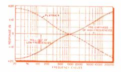
Fig. 2—An artificial response inserted into the recording characteristic is indicated by the solid equalization curve. The broken curve shows the playback equalization necessary to obtain true sound reproduction.
