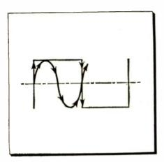
Fig. 4—A second harmonic cannot "ring in" a square wave since the action of the leading edge is cancelled by the trailing edge.
