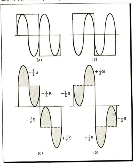
The voltage of the third harmonic may be observed by the area changes in Fig. 6c. When combined in-phase with the square wave, the area change is "2/3S", since the positive and negative sides of the wave both contain two "1/3S" areas that cancel each other, leaving a single "1/3S" area increase in both the negative and positive sections of the square wave.
