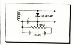
Fig. 4—A semicap silicon diode is used as a variable capacitor in a tuned circuit.
