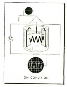
Fig. 1-A self-energized method of excitation can be achieved by using two diodes which block a-c to the grid, allowing a pulsating d-c potential of the proper polarity.
