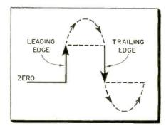
Fig. 2—Ringing of an LC circuit is sustained by the same leading and trailing edges.
