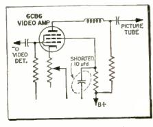
lig. 2—An intermittently shorted screen bypass capacitor causes a negative picture.
