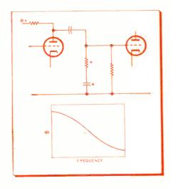
Fig. 6—High frequency slope circuit determined by the value of asterisk components.
