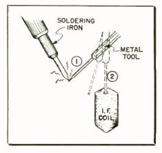
Fig. 1—Heating an alignment tool unfreezes wax dropped into i-f cores during production.
