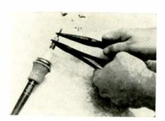
Proper tiplet removal is accomplished by firmly grasping the iron barrel and tiplet with pliers and rotating the tip out.
