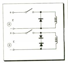
Fig. 5—Circuit choices are available when using selenium diodes as contact protectors. Circuit (B) is used with an a-c supply voltage.
