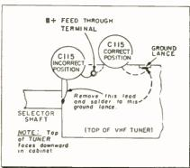
interference beats can be caused by capacitor C115 (0.039  $\mu$ f) in Fig. 2 being improperly grounded. A visual check of this capacitor can be made by removing the VHF tuning knob and observing the front edge of the tuner through the opening. If the capacitor is grounded at the front edge of the tuner instead of the ground lance located on top of the tuner, midway between the front rear, it should be unsoldered and grounded to the proper location.— RCA Service Company, Camden, N. J.
