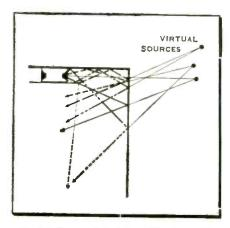
Fig. 2—Frequencies above 150 cps bounce off rear and side walls to cover room with stereo effect. Sound acts as if coming from virtual image source behind wall.
