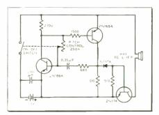
Efficient pulse generator with pitch control. Circuit parameters are adjusted to yield maximum acoustic output with minimum current.
