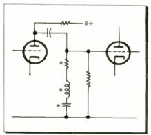
Fig. 8—Circuitry counterbalances unwanted rise in the middle of a frequency response. Components with \* determine frequency.
