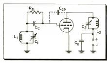
Fig. 2—Schematic shows impedance coupling between two audio vacuum tubes.
