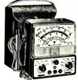
NOTE: The line cord is used only for capacity measurements. Resistance ranges operate on self-contained bat-teries. FEATURES: • A built-in Isolation Transformer automatically isolates the Model 80 from the power line when capacity service is in use.
