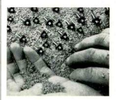
inclusive. Designations on the studmount types are IN332 through IN337; IN339 through IN346; IN348; IN349; IN550 through IN555; IN607 through IN614, and IN607A through IN614A. PIV ranges up to 600 v., currents to 500 ma. General Electric Semiconductor Products Dept., Syracuse, N.Y. (ELEC-TRONIC TECHNICIAN 5-45)
