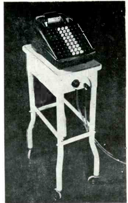
Fig. 5—Power and ground lines are permanently connected to this noise source to avoid compromising the work of the filter, after the technician leaves the job.
