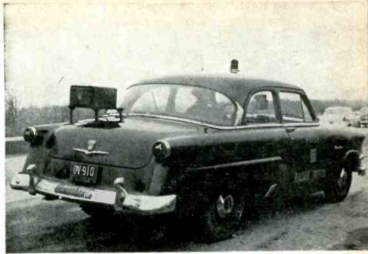
Patrol car is positioned as close to the road as possible to avoid parallax error.
