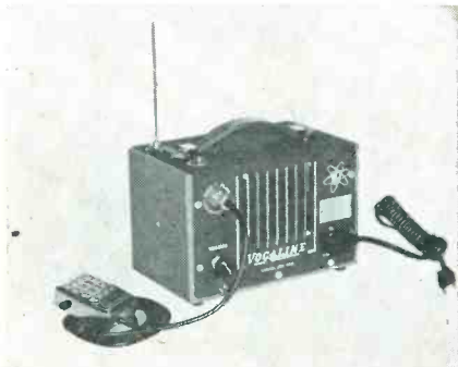
Fig. 2—Class B, 2-way radio operates at 456 mc, range varies from a few hundred yards to as much as 10 miles over land.
