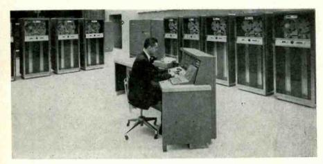
Electronic data processing machine combines the ability to calculate at unbelievably high speeds with a vast electronic memory. A central processing unit performs calculations in millionths of a second, and has the ability to make logical decisions.
