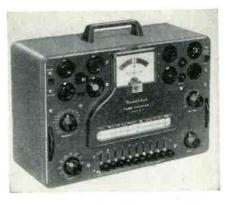
Tube condition is indicated on illuminated 3½" meter. Neon bulb shows filament continuity and leakage or shorts between elements. Roll chart runs freely. Suited for portable applications. \$39.95. Heath Co., Benton Harbor, Mich. (ELECTRONIC TECHNICIAN 10-11)
