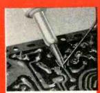
Slotted De-Soldering Tiplet flows solder neatly to replace, repair and rebuild circuit lines.
