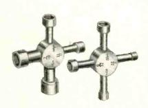
TWIN-X WRENCH SET (ETR-752)—designed and built expressly for TV-radio repairwork. Replaces eight hex-head socket wrenches  $\frac{3}{2}$ " to  $\frac{1}{2}$ ". Sizes are clearly marked for quick selection. Hollow shafts permit wrench to grip the nut over protruding end of bolt. Chromeplated case-hardened steel—will stand up in long, hard service.
