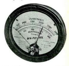
Fig. 5—When the conventional movable indicator, in the meter relay, contacts a fixed but adjustable arm, the load circuit is completed.
