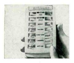
REMOTE CONTROL is nothing new, but the RCA Wireless Wizard control at left is different. This transistor-powered unit controls color TV sets, including "color" and "tint." Other RCA TV design trends are the use of surge resistors and power transformers in all sets, portables with 3 i-f's instead of 2, and a tetrode tuner instead of pentode. 90-day parts & labor warranty was announced. At right is prerecorded 4-track stereo tape cartridge and recorder, which eliminates reel threading.
