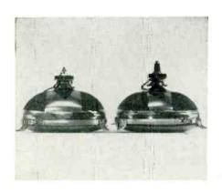
THE "SLIM LOOK" in TV set design gets an extra boost from Philco's development of the SF 110° tube shown at left. This new 21-incher is almost 2 in. shorter than the standard 110° tube beside it. The "Separate Look" is another innovation of the company's Predicta series, as shown by the swivel-mounted tube atop the chassis at right. The chassis slides out like a file drawer for easy access. Another variation allows wired CRT to be moved 25 ft. from the chassis.
