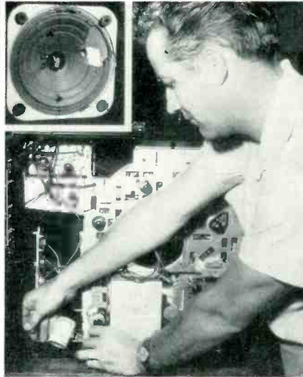
Roach Hive placed inside TV set prevents infestations. Note damaged speaker cone.
