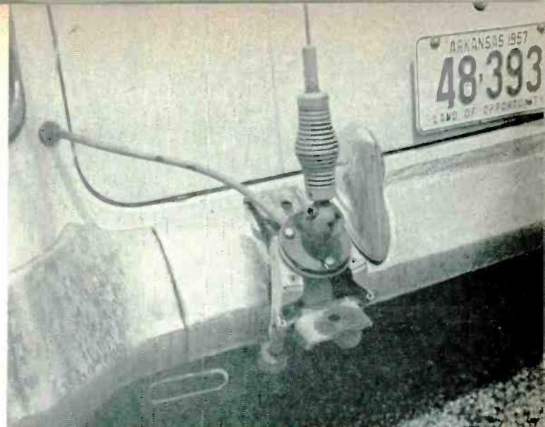
Fig. 5—Bumper-clamp type trailer hitch modified to hold a standard two-way radio antenna. It is easy to make and very sturdy.
