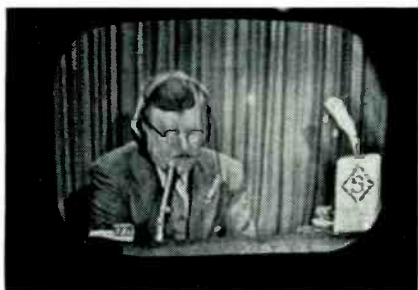
Fig. 2—"Sporadic E" starting to build up on a low-band channel (signal normally good) near New York. Interfering transmitter was operating on the same channel in Missouri.
