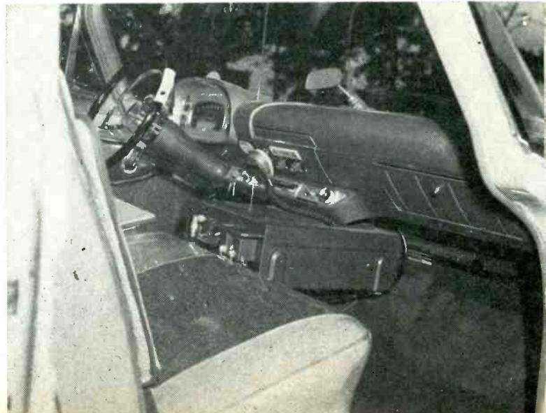
Fig. 2—Front seat installation. Radio dummy plate used to hold control head and microphone. Eliminates drilling new holes.
