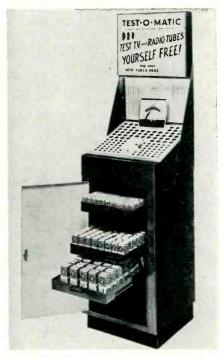
Do-it-yourself TV set owners can check their own tubes on this machine made by Shell Electronic Mfg. Service operators install a route of them in high-traffic stores.
