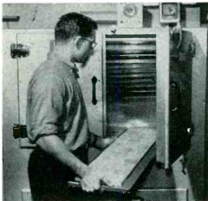
Electronically controlled fusion chamber receives 3,000 individual diamonds resting in sockets atop 3,000 steel pins. This bonding process which results in joining steel to diamonds is the first step in the automated production of Walco phono needles.
