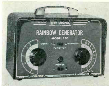
Fig. 2—Rainbow generator provides 1 to 8 complete vertical rainbows via linear phase sweep. Has facilities for crystal control.
