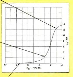
Plate current characteristics, shown on this typical test curve, are carefully controlled by the "fixed bias" test, assuring good performance and stable AGC functioning over a wide range of TV signal conditions.
