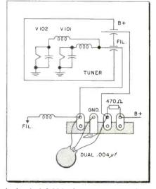
Leaky dual 0.004  $\mu f$  capacitor caused hum.
