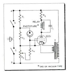
Fig. 4—Increase in light starts relay action
