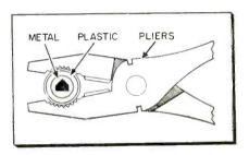
Fig. 3-Pliers shapes collar during cooling.
