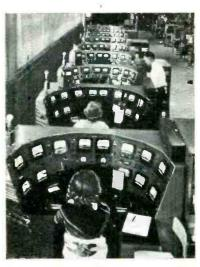
Dynamic TV set conditions are set up in these test bridges making the "fixed bias" test a true measure of how the tube will perform in TV sets encountered by you in the field.
