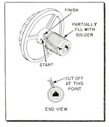
Fig. 2-Wire is wound, twisted around collar.
