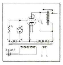
Fig. 3-Basic a-c operated amplifier circuit
