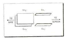
Fig. 3—For maximum sensitivity use the pair of deflection plates closer to the base of the CRT. Tube may be rotated to allow proper waveform display.
