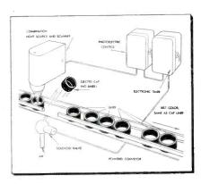
Fig. 7-Detector ejects gasket-less caps
