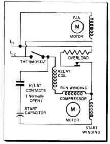
Fig. 2—Initial surge current through the relay coil momentarily closes the normally open contacts and activates the start circuit.
