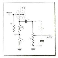
Fig. 4—Lower value of R<sub>4</sub> improves frequency response. Approximately 1500 to 3000 ohms.
