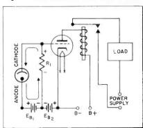
existing between the tube elements. Increasing the light intensity or the tube potential will cause the phototube current to increase up to saturation.
