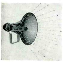
Fig. 2-Pattern widened by split-air column.
