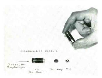
Transistor "radio pill" which is swallowed by patient has been developed by Rockefeller Institute, New York VA Hospital and RCA for research in the human intestinal tract. It consists of an FM transmitter modulated by action of intestine fluid or gas pressures on the capsule's diaphragm. Rechargeable battery has 15-hour life. Frequency is 1 mc, and signal travels 1 ft.
