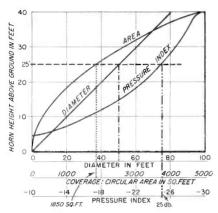
Fig. 5—Reflex radial characteristic chart. Projections from the intersections of the height above ground line ( ---) and the area, diameter and pressure index curves, indicate: area in sq. ft. ( . . . . ); diameter in feet ( ---); and pressure index ( ---) respectively.
