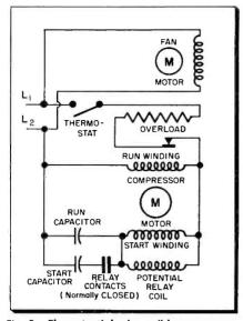
Fig. 3—The potential relay coil becomes energized and opens the relay contacts after compressor motor reaches 80% of its full speed. sufficient freon to enable normal cooling.
