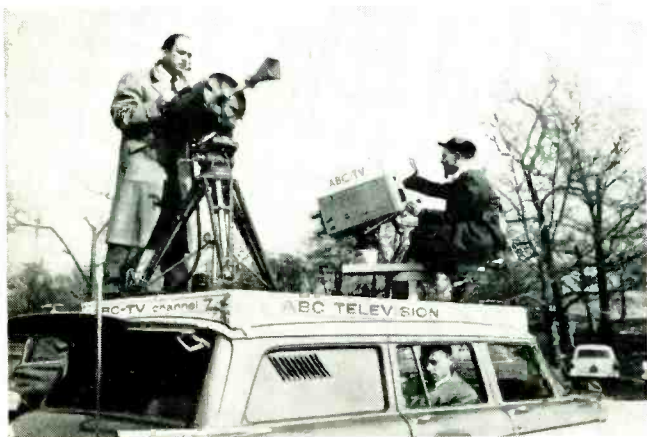
Microwave transmitter at left uses Narda horn instead of dish-type parabolic antenna to relay TV camera pickup from "crash unit" to main station. For parades and emergencies, the small horn allows increased flexibility while the camera is in motion.
