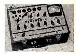
20,000 ohms/volt DC, 5000 ohms/volt AC, and measures current as low as 1 microampere, voltages up to 5000, ohms to 10 megs. Bulletins on these instruments available from Hickok Electrical Instrument Co., 10514 Dupont Ave., Cleveland 8, Ohio.—RADIO & TELEVISION RETAILING.
