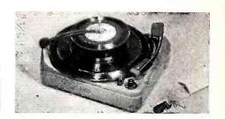
with interchangeable G.E. Variable Reluctance cartridges. Either cartridge (microgroove or regular) snaps easily into the tone arm, and they are color-coded. The model 100 is an amplified 3-speed unit with 3 tubes and a duo-needle reversible cartridge and is priced to retail at \$34.95. V-M Corp., Benton Harbor, Michigan.—RADIO & TELE VISION RETAILING.
