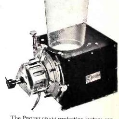
The Proteloram projection system consists of a specially developed 2½" projection tube, an optical box with focus and deflection coils, and a 25 kv regulated power supply unit. Compactness and flexibility make possible large-picture television in average size radio-phonograph consoles, consolettes and table model television receivers.
