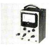
is calibrated for a 600-ohm circuit based on a reference level of 1 milliwatt. This VTVM measures up to 1000 volts AC or DC on a 5range linear scale and up to 100 megohms in 5 ranges. This kit is complete with tubes and instructions for assembly. Radio Kits Co., 120 Cedar St., New York, N. Y.—RADIO & TELE-VISION RETAILING.
