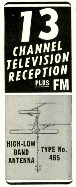
\* Definitely a "must" with television set owners who want to see ALL the available TV programs. TACO Type 465 High-Low Band Antenna handles TV Channels 7 to 13 as well as the easier 1 to 6. Also topperformance FM. Separate top section, adjustable for any direction, does the trick. Quarter-wave length jumper automatically applies either antenna to receiver. Aluminum sectional mast and clamps for mounting. Biggest value yet!
