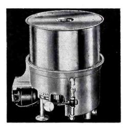
own motor-operated centrifugal pump, used to recirculate the water, drawing it through the bottom from the fine strainer which collects refuse. 2½ gallons of water required to fill wash reservoir. Two baskets are furnished, one for dishes, one for glasses and silverware. Optional equipment includes electric immersion heater and thermostat control. The Jackson Dishwasher Co., 3703 W. 93 St., Cleveland 5, O.—RADIO & Television RETAILING
