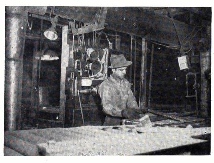
Above, mixer position is key point. Operator must be able to call quick instructions to scrap room, scales and rollers without ceasing supervision of material flow. Heavy layer of grit surrounds speakers, but can't get through reflex baffle.
