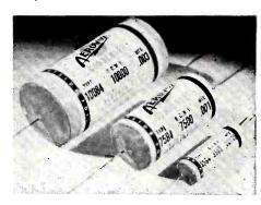
Paper tubular capacitors now being made by Aerovox Corp., New Bedford, Mass., for TV, oscillograph, other cathode ray and electronic circuits have voltage ratings up to 10,000 volts d-c working. Oil impregnated and wax filled, the Series 8 have from .001 to .05 mf.
