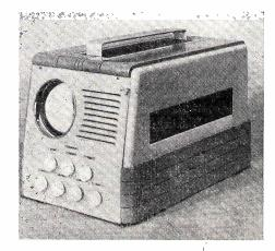
A new television kit, shown here in specially designed cabinet, is offered by Espey Mfg. Co., Inc., 528 E. 72nd St., New York 21, as particularly suitable for servicemen, experimenters, students, etc. Espey plans to market only the basicit; buyers get remaining parts themselves. It has a 3" picture tube, miniature tubes, simplified superhet circuit.
