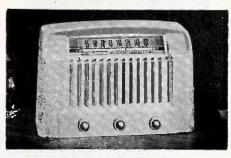
Model 300W table superhet tuning 540 to 1620 kc. Tuned r-f amplification, ac-dc, 3-gang condenser, 4 by 6 Alnico oval speaker, improved automatic volume control. Five tubes, including multi-purpose plus rectifier. Super-signal antenna, jack for phono. Concealed handle molded into cabinet. "Brite-Lite" dial. One-piece plastic cabinet—ivory finished. Measures 1234" wide by 8½6" high by 8¾6" deep. Bendix died Division, Bendix Aviation Corp., Baltimore 4, Md.—RADIO & Television RETAILING
