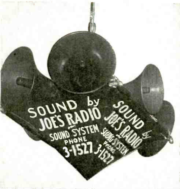
More prominent than the game itself is the 6-speaker basket, part of Joe's rental system.
