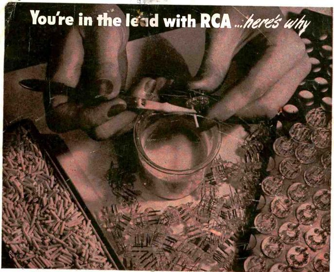
Cementing ceramic insulator to miniature tube button stem—one of the many delicate operations in making an RCA tube that calls for unusual skil.
