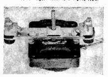
motor is one of three types to be discussed now. This unit has been used in many record changers, and is generally mounted in a cradle, insulated from the rest of the equipment by two rubber bushings on the mounting flanges.
