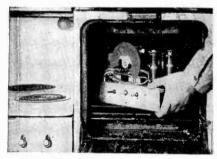
Chassis heat should be comfortable to touch.
