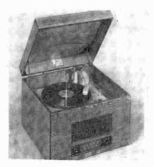
Model 202 radio-phonograph table unit, ac-dc superhet, 6 tubes including rectifier, automatic record changer playing twelve 10" or ten 12" discs. Tunes 550 to 1700 kc, built-in loop antenna, automatic volume control, slide rule dial, Alnico 5 PM speaker. Cabinet of walnut veneers measures 12" by 15½" by 16½". Weighs 27 lbs. Apex Radio & Television Corp., 192 Lexington Ave., New York 16, N. Y.—RADIO & Television RETAILING
