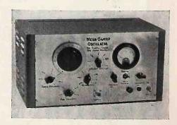
The Mega-Sweep oscillator has a carrier frequency range from 50 kc to 500 mc, with an adjustable sweep from 30 ke to 30 me broad. An output of .1 volt at a 50-ohn level is controlled by a continuously variable attenuator. The amplitude modulation while sweeping is kept to .15 db per megacycle. Kay Electric Co., East Orange, N. J.—RADIO & Television RETAILING
