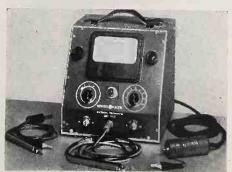
measured on the 1, 3, 10, 30 and 100 volt scales, while a multiplier switch is used to increase the d-c range by 10 X. Four resistance ranges cover up to 100 megohms. General Electric Corp., Specialty Division, Wolf St. plant, Syracuse, N. Y.—RADIO & Television RETAILING
