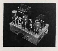
in the frequency range from 40 to 10,000 cycles, within ±1 db. Push-pull 6L6-G tubes deliver the output into impedances of 4, 8, 15, 250 and 500 ohms. Filament and plate voltage is also provided for an external 4 or 5 tube preamplifier. Pan American Electric Co., 132 Front St., New York 5, N. Y.—RADIO & Television RETAILING
