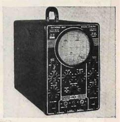
range from 20 to 50,000 cycles uniformly within 20%. There is provision for intensity modulation. The input impedance of the vertical plates are 5 meganisms. ohms at 50 mmf direct, and 1 megohm at 40 mmf through the amplifier, while the horizontal impedances are 5 meg-ohms at 60 mmf direct, and 5 megohms at 40 mmf amplified. Allen B. DuMont Laboratories Inc., 2 Main Ave., Passaic, N.J.—RADIO & Television RETAILING
