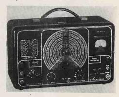
Model 1632 is an amplitude modulated signal generator covering from 100 kc to 120 mc in 10 ranges. The panel meter indicates the output of the multiplier and attenuator. Provision is made for internal mounting of a 1000 kc crystal, for heterodyne frequency calibration. Air trimmers, permeability tuned coils and a voltage regulator tube are included for stability. Triplett Electrical Instrument Co., Bluffton, Ohio—RADIO & Television RETAILING
