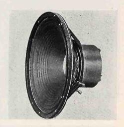
diaphragm for generating and dispersing the highs. The 3" voice coil is edgewound with aluminum wire, and has an impedance of 10 ohms. The Alnico V PM speaker is rated at 18 watts audio. Altec Lansing Corp., 250 W. 57th St., New York 19, N. Y.—RADIO & Television RETAILING
