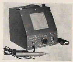
Model 200 uses a PM speaker connected to a high gain amplifier which reproduces r-f, i-f or audio signals. A low value of capacity coupling through the polystyrene probe prevents disturb-ance of the operating characteristics of the circuit under test, and operates to over 300 mc. Precision Electronics Inc., 641 N. Milwaukee Ave., Chicago, Ill.— RADIO & Television RETAILING
