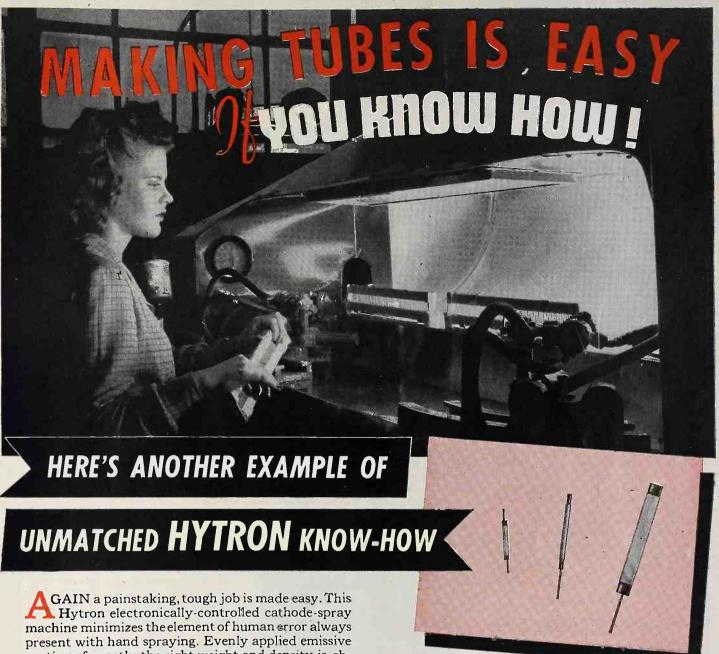
coating of exactly the right weight and density is obtained hour after hour. Number and speed of coating passes, distance from spray guns to cathode sleeves, and intensity of the spray are precisely controlled.
