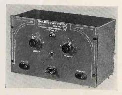
The "C" supply is variable from 0 to 75 volts with less than 7 MV ripple. 6.3 volts at 2 amperes is available for an unregulated a-c filament supply. Communication Measurement Lab., 120 Greenwich St., New York, N. Y.—RADIO 5. Television RETALLING. & Television RETAILING
