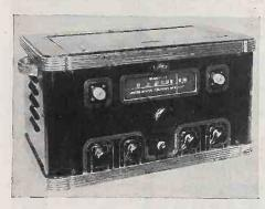
use. Separate crystal-controlled oscillators supply marker frequencies at 1 mc and 10 mc intervals. A heterodyne or beat-frequency circuit is used, with a stage of amplitude limiting. Output voltage is from 30 microvolts to .1 volt, at an impedance of 100 ohms. Operates on 110v, 50-60 cycles. U. S. Television Mfg. Corp., 3 W. 61 St., New York 23, N. Y.— RADIO & Television RETAILING
