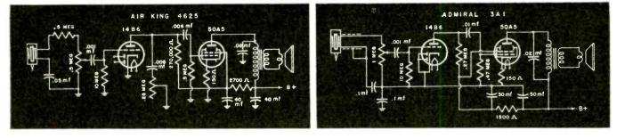
Essentially the same circuit is employed in most 2-stage phone amplifiers. Differences above are for tone control in Alr King, and use of radio or
