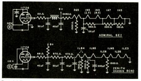
Two typical filament circuits. Purpose of many resistors is to keep filament current to 50 milliamperes by by-passing the significantly extra current added by plate circuit.
