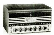
than .5% at the 12-watt level. An overall gain of 96 db is maintained from 20 to 20.000 cycles.  $\pm$  1db. Hum and noise level is — 40 VU. Two  $\frac{1}{2}$  megohm inputs are provided, with variable-timing volume expander and separate low and high frequency equalizers. The 15 output taps range from 1 to 500 ohms. Amplifier Co. of America, 396 Broadway, New York, N. Y.—RADIO & Television RETAILING
