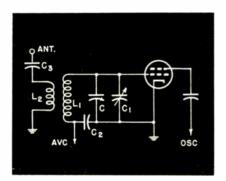
Adjusting trimmer C1 and padder C2 should result in good alignment at three points.
