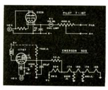
Less frequent arrangements. Adding 7500  $\Omega$  resistor boosts filament voltages in bottom circuit.
