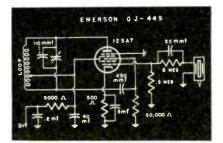
Common practice of wireless players is to use grid \$1 for modulation. Oscillator circuit inductance is used here as a radiating loop.
