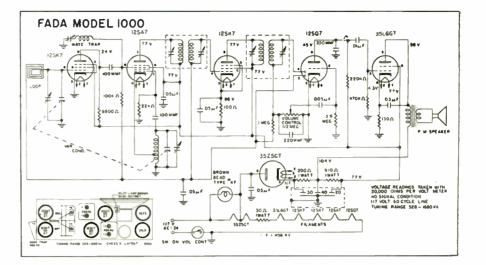
**FADA MODEL 1000** uses a tuned r-f stage in which the loop is the coil. Although the mixer grid circuit is tuned, the frequency of the resonant circuit is adjusted to 456 kc, the i-f value. Since the circuit is series resonant across the mixer grid to ground, it effectively eliminates i-f signals, either from feedback or external interference such as airplane beacons.
