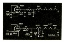
In old sets, removing tube Z damaged 25-v filter. Z, replaced, killed other tubes.
