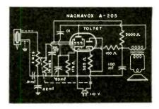
High value of capacity is required for single filter capacitor. Simplicity of this type of circuit is reflected in infrequent servicing.
