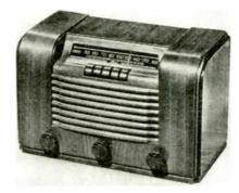
Model R-1238 table model receiver. ac-dc, tunes 550 to 1700 kc. Six tubes, automatic tuning and volume control. Wood cabinet—walnut finish. Measures 131/2" wide, 83/4" high, 71/8" deep. Delco Radio Division, General Motors Corp., Kokomo, Ind.—RADIO & Television RE-TAILING
