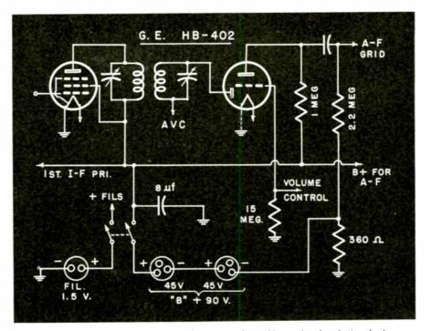
Straight battery portables use parallel filaments; main troubles are in tubes, battery leads.
