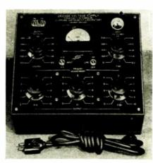
frequencies, up to 10,000 cycles, may be used in this instrument, which incorporates a transformer having a tapped primary and secondary. A Weston Model 476 meter is placed in the secondary circuit, with a single red line to indicate proper primary voltage adjustment. Clippard Instrument Laboratory, 1440 Chase Ave., Cincinnati 23, Ohio.-RADIO & Television RETAILING
