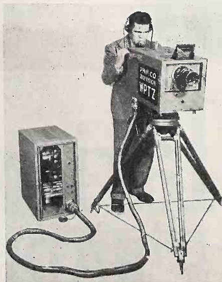
W. A. Howard demonstrates the new 35-lb. Philco camera, with auxiliary "suitcase" unit.
