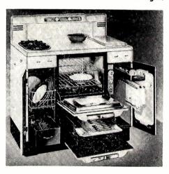
Broiler in roller bearing drawer. Several compartments for warming and storage. Dimensions: length 38", depth 26", overall height, 44½", height to cooking top 35½". The Tappan Stove Co.. Mansfield, O.—RADIO & Television RETAILING
