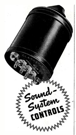
★ This compact, inexpensive, constant-impedance output attenuator (Clarostat Series CIB) will dissipate 10 watts at any selling. Operates noiselessly without distortion. It is highly recommended as an individual speaker control in a multi-speaker P-A system. Linear attenuation in 3 db steps up to 30 db, and then final step to infinity. Insertion loss is zero.
