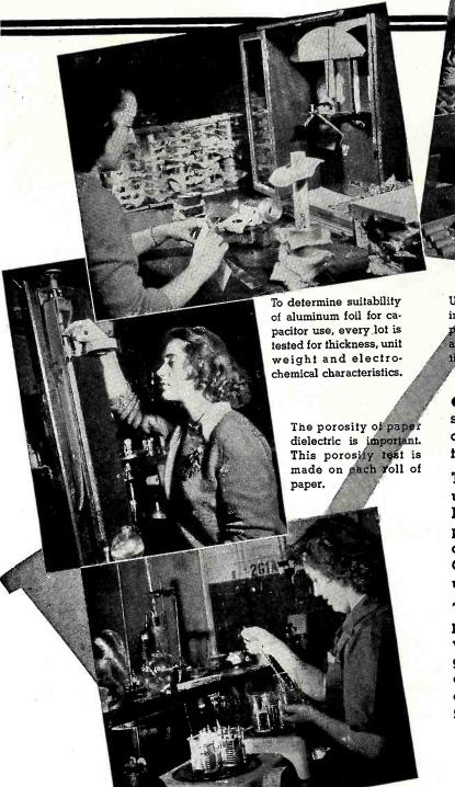
Uncased paper sections are checked prior to impregnation. Completed units are tested for capacitance, power factor, insulation resistance, terminal-to-terminal and terminal-to-can, as well as for dielectric strength and tightness of seal.
