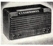
Model 6-506 uses dual-purpose tubes in 5-tube ac circuit. Permits use with
