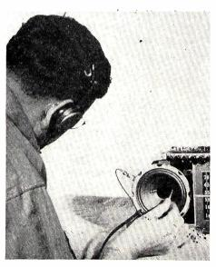
shown in illustration. If the voice coil is open, and no other troubles are present, signals will be heard in the phones when set is tuned to a station.
