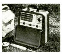
pedance loop aerial welt-sewed into cabinet covering to give greatest signal pickup. Tuned radio frequency stage with 3-gang condenser. Alnico No. 5
