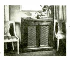
fiers and tuning eye. Optional FM chassis has 8 tubes including tuning eye and rectifier. Set has two 12" Duosonic speakers and 8-station pushbutton tuning. Dimensions are 34" wide, 19½" deep, 38½" high.
