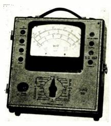
volts, at 1000 ohms per volt; dc amps, 0-10; ac amps, 0-0.5-1-5-10; dc milliamps, 0-1-10-50-250; dc microamps, 0-50; ohmsmegohms, 0-4000-40.000 ohms, 4-40 megohms. Triplett Electrical Instrument Co., Bluffton, Ohio—RADIO & Television RETAILING
