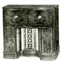
Model 106CR radio-phono console combination has floating jewel tone system, Seeburg "single control" record changer. Plays ten 12" or twelve 10" records. 6 push buttons for automatic tuning. Has solid top cabinet with drop-front doors. Two records compartments at sides of recessed grille. Set has 10 tubes and measures 37" high, 401/8" wide, 181/8" deep. Crosley Corp., Cincinnati 25, Ohio—RADIO & Television RETAILING
