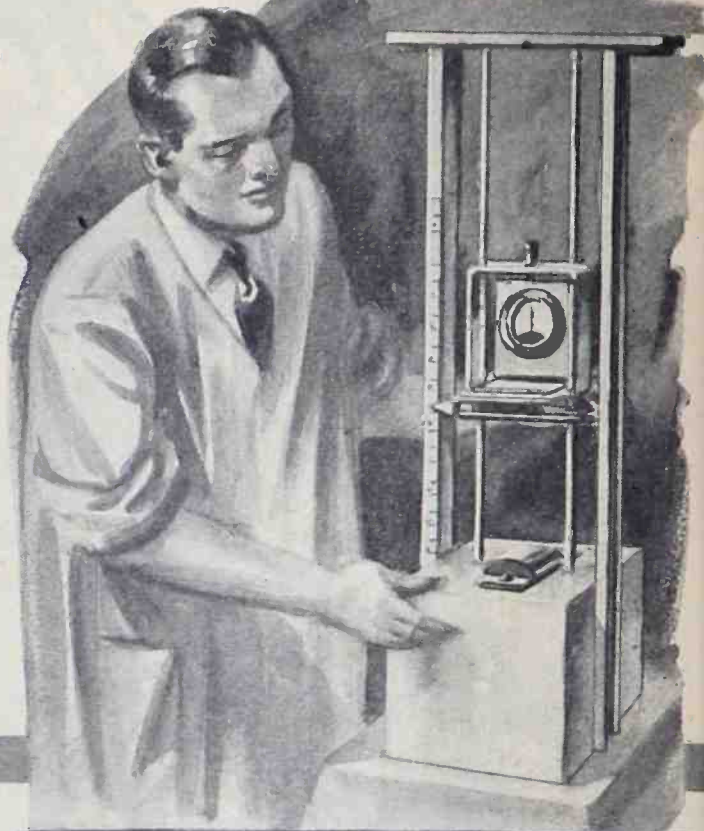
Simpson Shock Test —Instrument is mounted in sliding carriage, and dropped against bottom plate. Vertical scale permits shock of impact to be computed in multiples of g, the acceleration of gravity.
