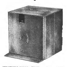
**STRUTHERS-DUNN TIMER.** Type PSEH-1 made in both AC and DC types. Closes contacts at end of predetermined delay interval after power has been applied or after reset of a momentary impulse. Double-pole double-throw relay provides load circuit flexibility. Struthers-Dunn Inc., 1321 Arch St., Philadelphia 7, Pa.—RTR.
