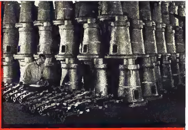
Right: Castings at the Norge plant prior to machining into pedestals for Mark IV Oerlikon gun mounts.
