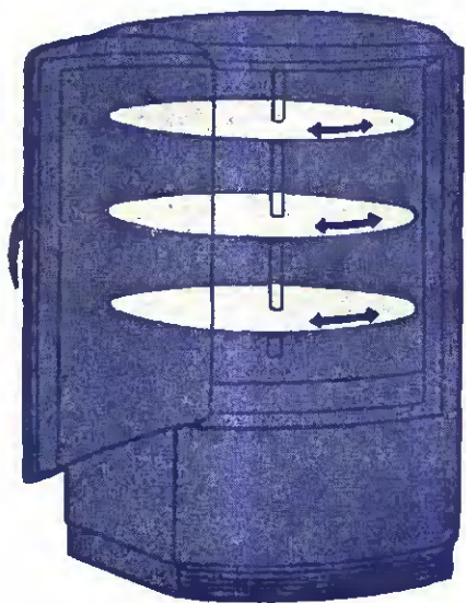
Note: This sketch of refrigerator, eliminates all sections in order to show clearly the revolving shelves.
