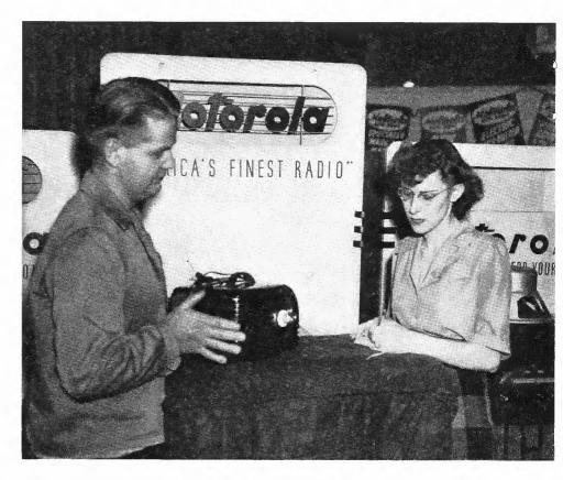
Above, Miss Gould meets a customer and takes the data on the set to be repaired. Below, Mr. De Young checks the set and finds that the trouble is noisy I.F. coils. At right, Miss Gould solders in the new coil and finishes the job by putting the chassis back into the cabinet.
