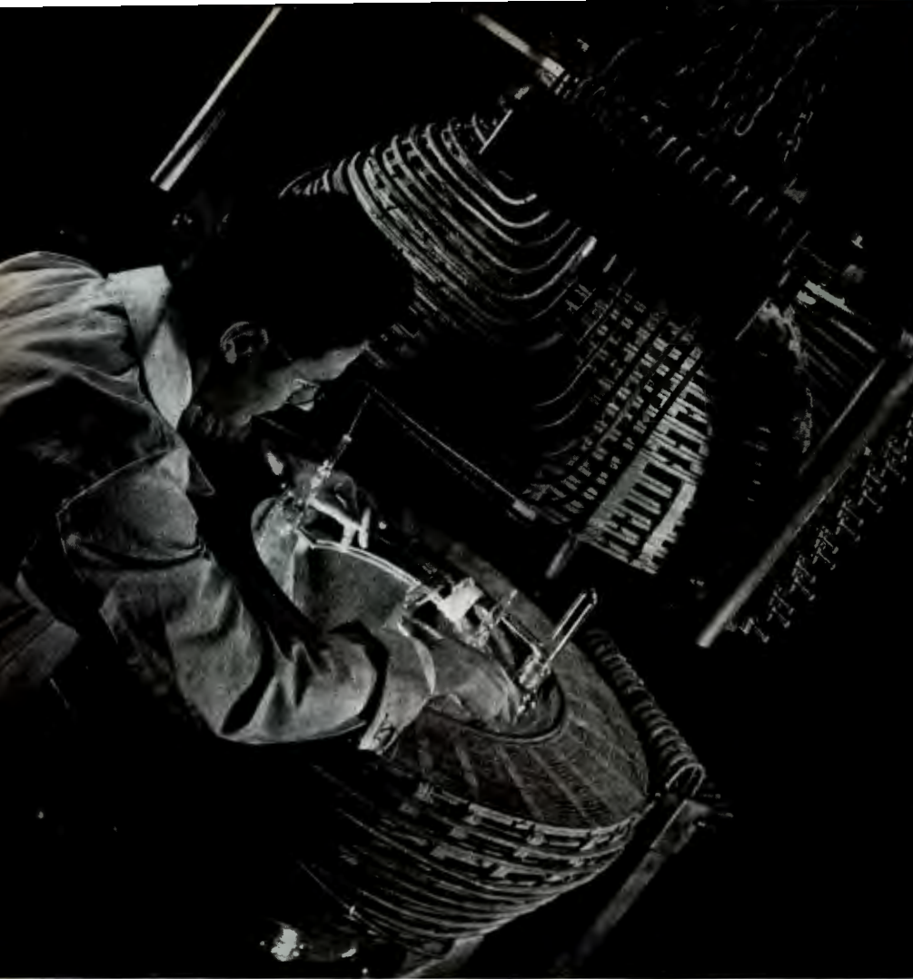
The electronic atom-sorting machine at the left illustrates the kind of research which keeps the new industry moving ahead. It's really a mass spectograph with magnetic field coils surrounding the atom-sifting tube in the center.
