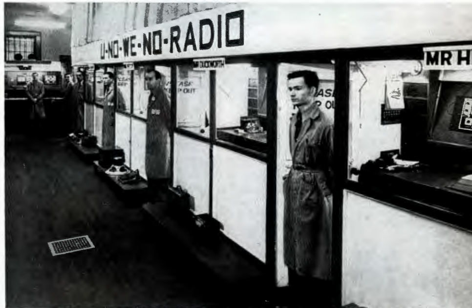
The "mass production" service methods at the Dixie Radio Supply Co., Columbia, S. C., make the best possible use of technical personnel. These men do only production work laid out for them in their individual booths; they can repair 70 to 100 sets a day.
