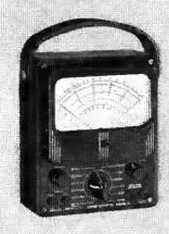
Here is a typical example of Simpson leadership. At 20,000 ohms per volt this tester is far more sensitive than any other instrument in its price range—covers a wide, range of unusual conditions which cannot be checked by ordinary servicing instruments. Six voltage ranges—0.2.5, 10, 50, 250, 1000 and 5000 V—both AC and DC. Current readings from I microampers to 500 miliamperes. Resistence readings from 1/2 ohm to 10 megohns. Five decibel ranges,—10 to +52 DB.
