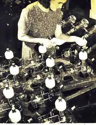
High-power radio transmitting tubes for U. S. Navy, being checked by Westinghouse girl inspector.
