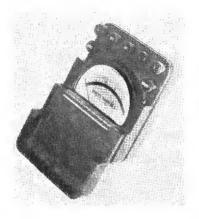
WESTINGHOUSE P-14 PORTABLE AC-DC INSTRUMENT for general field service, embodies both single and multiranges for measurement of ac volts, amperes and milliamperes, dc volts, amperes, milliamperes and micro-amperes. Insulated and magnetically shielded molded case. Available with or without covers. Scale length is 3.2 in. ac and 2.8 in. dc with accuracy of + or -1 per cent of full scale. Mirrored dial, knife-edge pointer. Westinghouse Elec. & Mfg. Co., E. Pittsburgh, Pa.—RRT.
