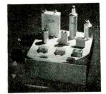
**SOLAR** TYPE XJ high voltage filter capacitors provide wide range of capacities in DC voltage ratings from 6,000 to 25,000. Heavy gage steel containers are welded oil tight and hot tinned. Wet process porcelain insulators. Vacuum treated mineral oil impregnant assures low leakage current and negligible capacity change over a wide range of operating temperatures. Illustration shows contrast in size between XJ and smaller capacitors on it. Solar Mfg. Corp., 586 Ave. A, Bayonne, N. J.—RRT.
