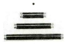
**WESTINGHOUSE** SECTIONAL RE-SISTOR—Individual, hermetically sealed units wire wound around a ceramic spool, with values of from 0.25 to one megohm, rated current of 1 MA. Dimensions are 13% in. x 11/4 in. diameter per section. Ad-Jacent sections are wound in opposite directions to obtain non-inductive resistance. Ends are tapped with a 10-32 thread and connected electrically and mechanically by a screw stud. Available in 7.5, 15 and 30-kv. sizes. Westinghouse Meter Division, Newark, N. J.—RRT.
