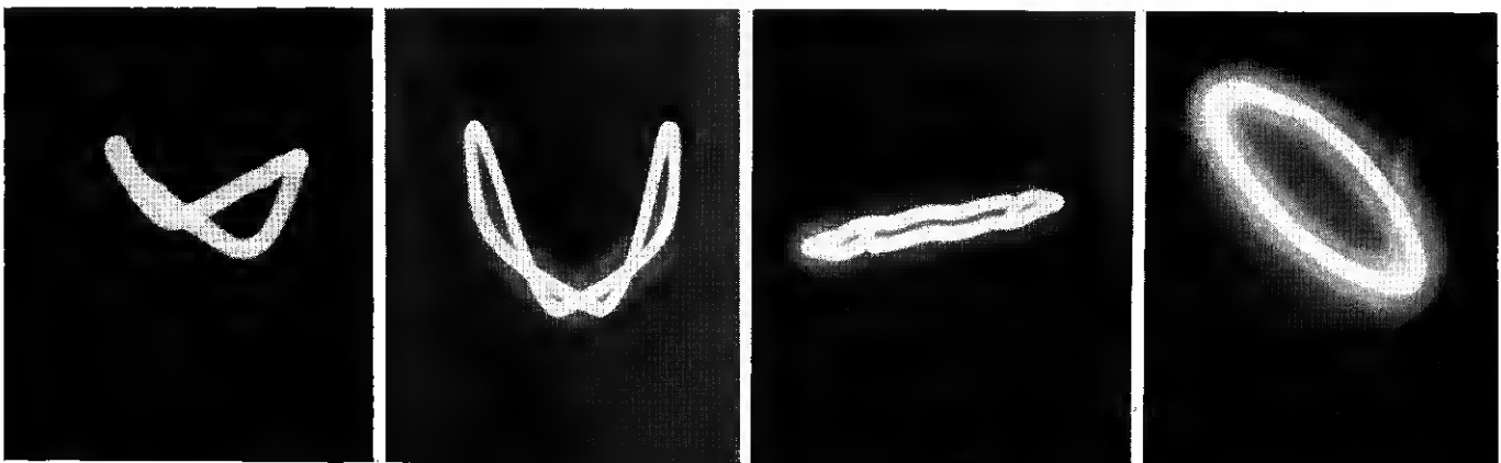
Fig. 4— A B C D Actual hum patterns due to different causes referred to in text. Pattern A is 60-cycle hum due to faulty tube cathode. B is the 120-cycle hum of about normal intensity. A bad case of 120-cycle hum is shown in C. D is the one-loop 60-cycle hum of half-wave power supplies.
