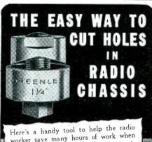
worker save many hours of work when cutting holes for sockets, plugs, connectors, and meter holes in radio chassis. No tedious drilling, reaming, or filing is necessary. A cap screw is inserted in a small drilled hole, and the punch is easily forced into the die by a few turns of the cap screw with an ordinary wrench. Ten punches are available for cutting 34, 78, 1, 11/8, 15/3, 13/6, 11/4, 13/8, 11/2 and 21/4 inch holes. Write for more information.
