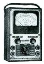
PRECISION MULTI-RANGE TESTER, series 834, hand, offers 18 voltage ranges, 0-12/60/300/600/1200/6000 in ac-dc and power output, at 1,000 ohms per volt; 4 current ranges, 0-12/12/60/600 mils; 3 resistance ranges, 0-5M/500M/5 megs; and 6 decibel ranges from —10 to +70 db. Precision Apparatus Company, 647 Kent Ave., Brooklyn, N. Y.
