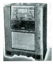
SENTINEL CONSOLE COMBINATION, model changer concealed in sliding drawer, plays 10 and 12-inch records in automatic sequence. Features illuminated record compartment, lifetime needle, and self-starting motor. Receiver is a 9-tube, 3-band ac superhet, tuning the standard broadcast, police and shortwave bands. Equipped with 12-inch speaker and pushbutton tuning. Sentinel Radio Corp., 2020 Ridge Ave., Evanston, III.
